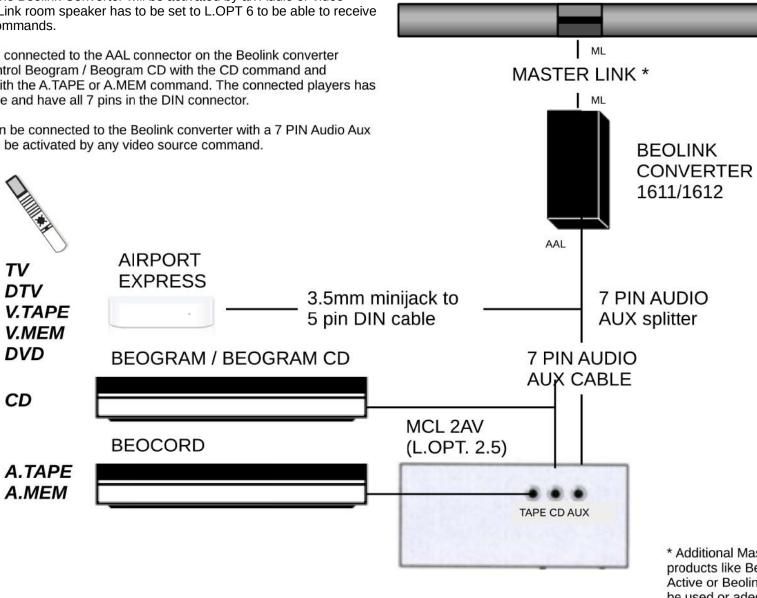
\* Additional Masterlink link room products like Beolab 2000, Beolink Active or Beolink Passive can also be used or aded in this setup The setup will not work if a Beosound with Masterlink is connected as Audio Master
